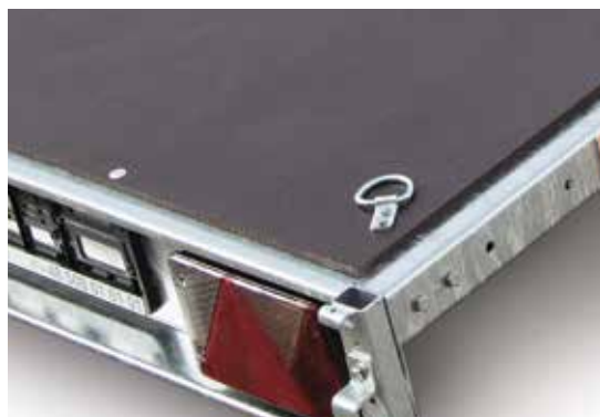
Internal hooks for cargo fixing screwed to the frame (from 235 SU and higher models up to 330 T)
