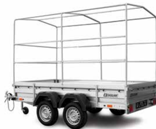
Light and easy to assemble frame construction for the tarpaulin
