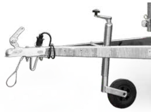
Supporting wheel mounted between drawbar beams
