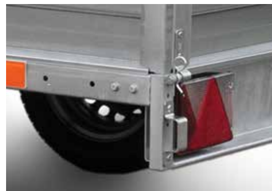
Easy storage in vertical position by using metal buffer
