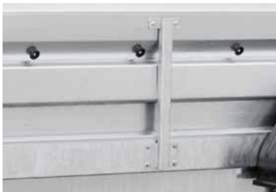
Four reinforcements of dropsides in standard (in models: 300 SU, 300 T and 330 T)
