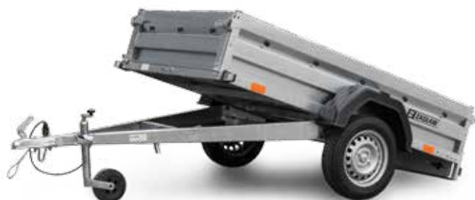
Tipping box-body – tilting function
