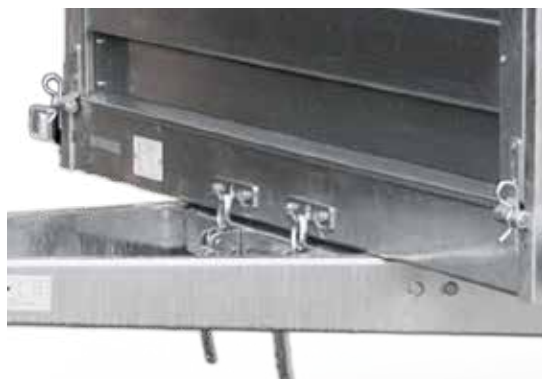
Tipping of box-body in 300 SU trailer is blocked with two hooks
