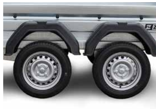
In tandem production there are used 2 axles of 750 kg loading capacity
