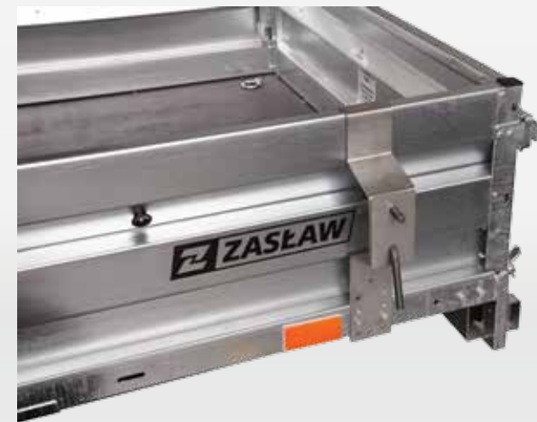
BRACKET OF SPARE WHEEL FIXING to a dropside
