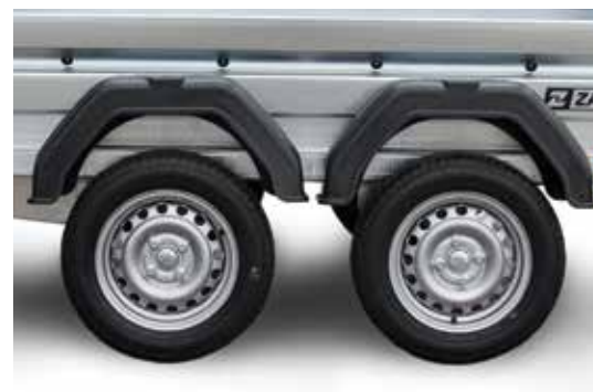
Two axles by KNOTT of 750 kg loading capacity are used
