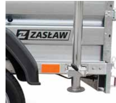
SIDE SUPPORTS useful when loading on a trailer which isn't coupled with a vehicle
